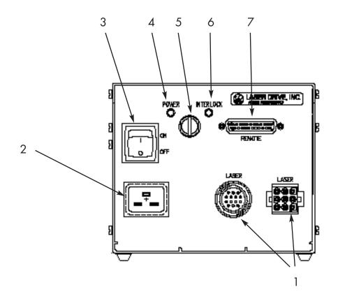
Figure 3.2 Front Panel Controls, Indicators and Connectors on the Laser Drive 8470 Power Supply
